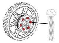
Step 4: Add two more pulley halves (am-2234-half) to the wheel.
