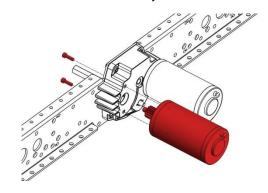
**Step 10:** Place the TB Mini onto the Inner Plate using the plastic studs to align the housing. The bottom flanged edge of the Inner Plate will be facing towards the gearbox housing.
