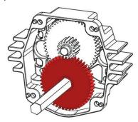
**Step 2:** Insert the TB Small Hex Shaft (am-0152) into R6ZZ bearing closest to the flat edge of the housing.
