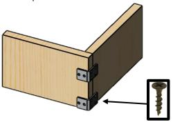
**<u>Tip:</u>** To ensure that bumpers designed to wrap around corners are rigid, it is recommended that the corner edge be strengthened with angled corner connectors such as am-3066 (not included).
