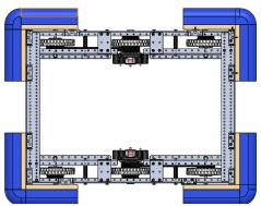
**Step 3:** Bumpers can either be made in straight sections or in sections that wrap around corners.
