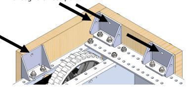
**Tip:** After drilling, it is helpful to label which bumper plank goes to each location on the chassis in order to easily re-attach later.
