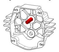
**Step 4**: Place the 16 tooth gear (am-0747) on the TB Small Hex Shaft with **flat side down.**
