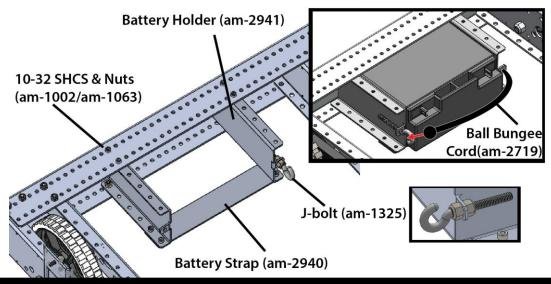
**Tip:** Batteries may vary slightly in width. In order to ensure the batteries slide in and out easily, place the battery between the holder rails and tightening the 10-32 screws with the battery in place.
