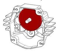
**Step 5:** Tap the 1/2" E-Clip (am-0206) onto the groove on the TB Hex Output Shaft (am-2566a).
