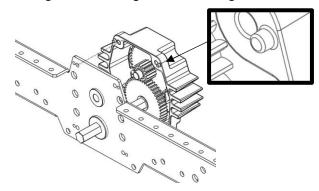
**Step 12**: Place two 5/16" Washers (am-1009) onto the CIM Motor shaft. Place the 2x2x10mm Machine Key (am-1121) into the keyway of the motor shaft. Push the 14 Tooth, 8mm Key Gear onto the shaft, to the face of the washers, while aligning the keyway with the machine key. Use a 7/16" socket to press the 8mm Retaining Clip (am-0033) onto the face of the gear.
