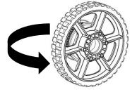
Step 5: Insert one 500EX Hex Hub (am-2568) into the pulley on one side of the wheel.
