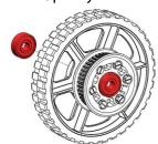
NOTE: Tighten the screws in a triangle pattern to ensure the pulley aligns evenly on the wheel.
