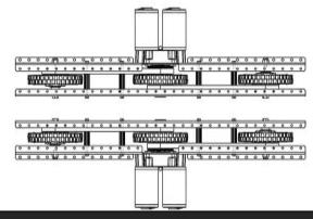
NOTE: The belts should be parallel to the side plates.
