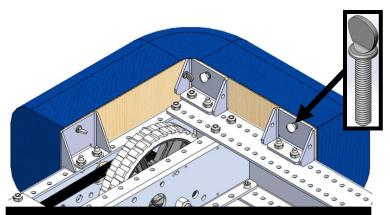
**<u>Tip:</u>** Alternatively you can use  $#10-32 \times 1.00''$  SHCS (am-1056) to attach your bumpers to the robot frame.
