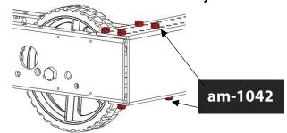
NOTE: The long chassis will use 6 screws and nuts per corner. The wide and square configurations will use 5 screws and nuts per corner.
