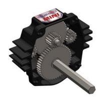
\*To change the drive speed of the AM14U3, different gear ratios can be used in the Toughbox Mini. The AM14U3 features a center wheel directly driven by a TB Mini Hex Output Shaft. To change the ratio and drive speed, the standard 16 tooth Small Cluster Gear and 48 tooth Large Output Gear will need to be replaced with two gears totaling 64 teeth. The higher the ratio, the slower the output speed.
